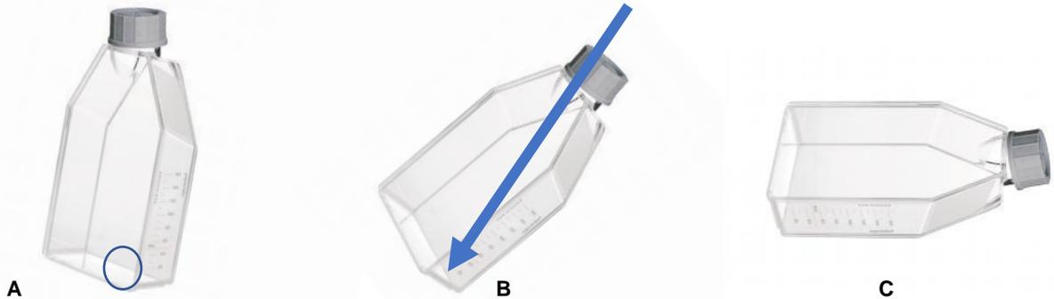
**Figure 2. Flask Orientations.** A. Location to place pipette tip when aspirating from a tilted flask. B. Dispense liquid onto the side of the flask(s) to avoid disrupting attached cells. C. When cells are seeded, lay flask(s) flat with media evenly covering the bottom surface.
